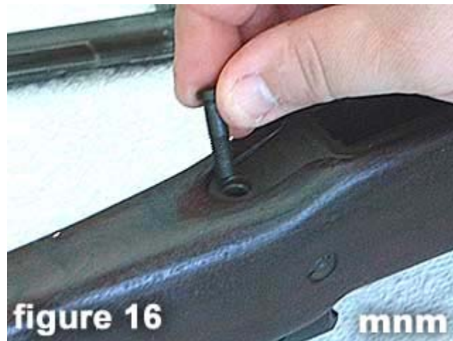
16) Remove the guard front screw .
