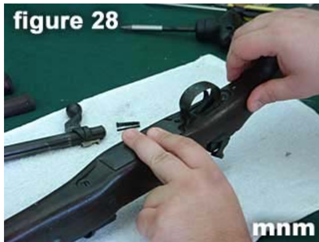
28) Snap floor plate catch in place.
