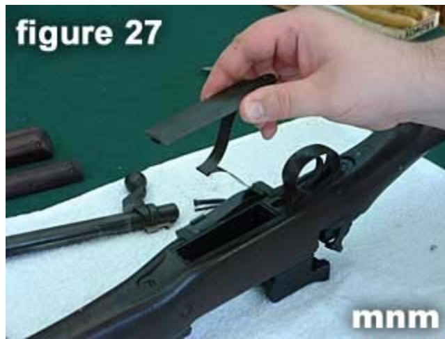
27) Place floor plate catch , magazine follower , and spring back into magazine well as show in figure 27 .
