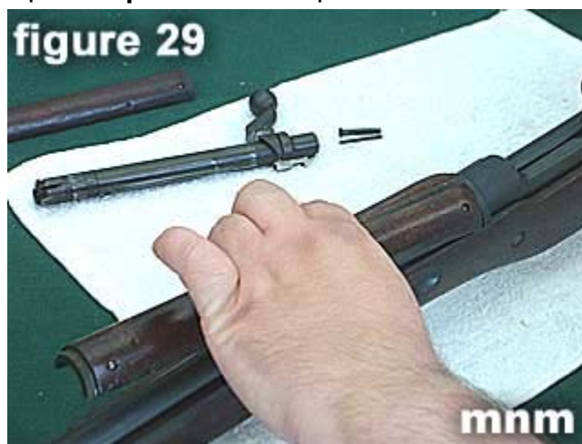
29) Slide the rear handguard into the handguard ring at the front of the receiver (as shown in figure 29 ).
