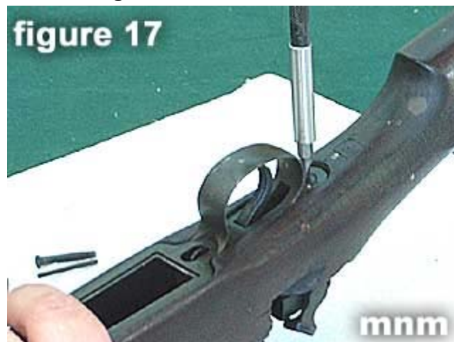
17) Unscrew the guard cover rear screw .
