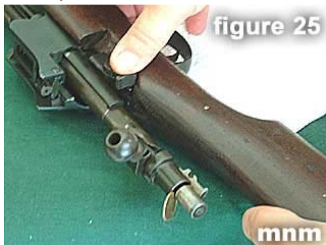
25) Make sure safety is engaged ( in safe position ).
