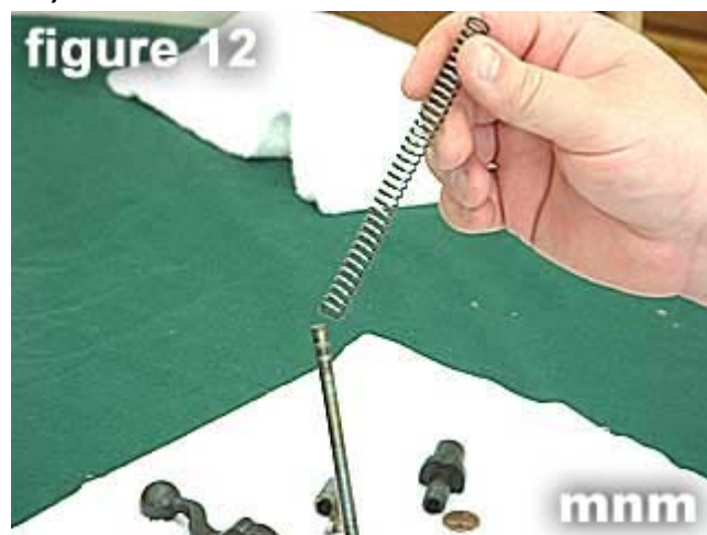
12) Remove the striker spring from the striker .
