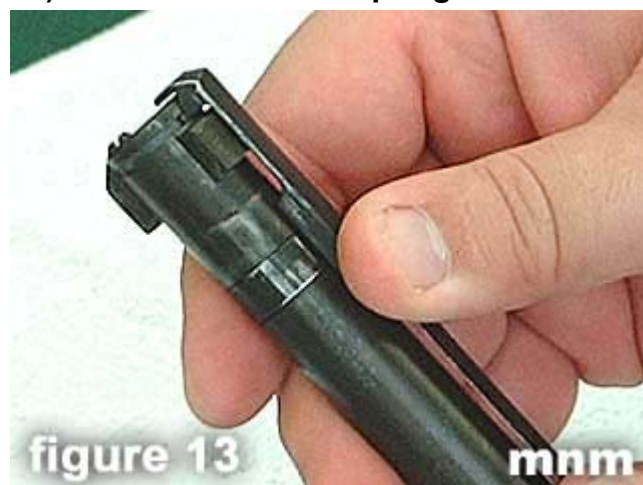
13) Turn the extractor ( clockwise ) so that it covers the gas escape holes in the bolt body .
