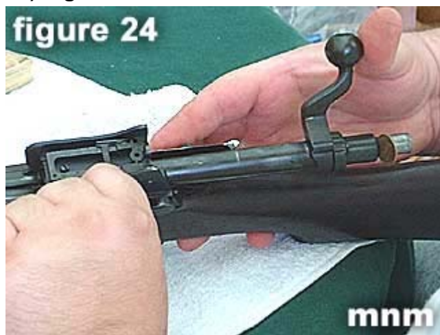
24) Align the bolt's extractor with right hand locking lug (solid - not slotted lug) on bolt and then insert into rear of receiver .
