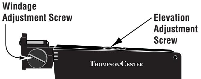
The T/C Fire Storm™ muzzleloader is equipped with a standard rifle rear sight (**Diagram “A” above**) which is adjustable for elevation by moving the elevation “blade” up or down to change the point of impact. To do this, turn the Elevation Adjustment Screw clockwise (as viewed from the breech end) to lower the point of impact, and counter-clockwise, to raise the point of impact.
