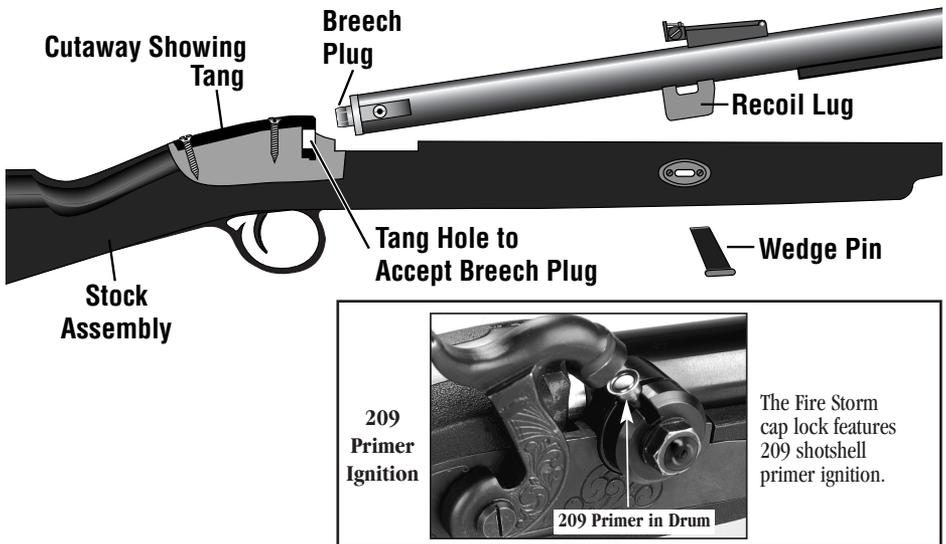
3. Tip the barrel down into the barrel channel in the stock. The recoil lug should fit neatly into the recoil lug receptacle slot in the stock.
