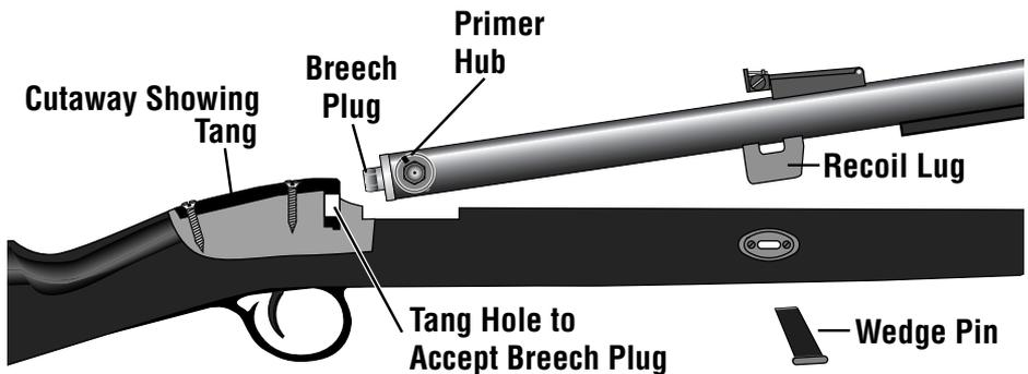
5. For those with the cap lock (209 version), further disassembly includes removal of the primer hub.
