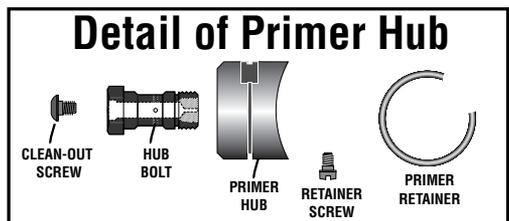
an anti-seize lubricant like Gorilla Grease before re-installing the hub to the rifle.
