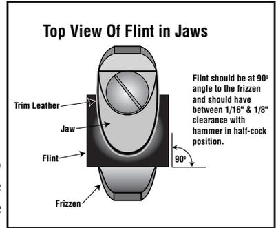
Make sure the flint is aligned in the jaws perfectly square, so that the edge of the flint is perfectly horizontal across the face of the frizzen. This will ensure maximum contact of the entire flint edge with the face of the frizzen.
