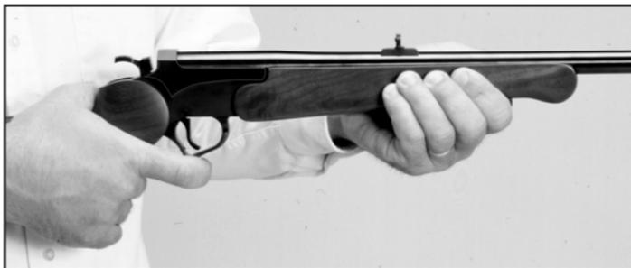
The Encore is a single shot, break open style rifle or shotgun. To open the Encore, grab the firearm with your left hand at the balance point on the forend. (Use right hand if you are left handed). With your other hand, pull rearward on the trigger guard spur with your trigger finger. Place your finger low on the spur for maximum leverage, and give it a fast sharp pull. Pull rearward and up at the same time.
