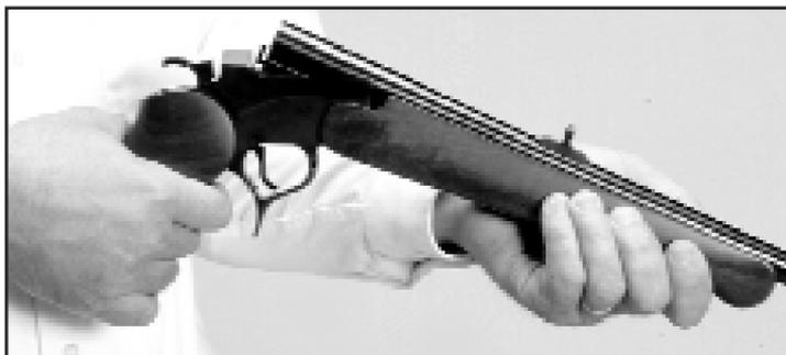
Pulling back on the trigger guard spur will allow the barrel to pivot downward. To close the Encore, pull the barrel upward while securely holding the rifle grip of the Encore stationary with your right hand. Practice opening and closing the Encore before attempting to load and fire this firearm.
