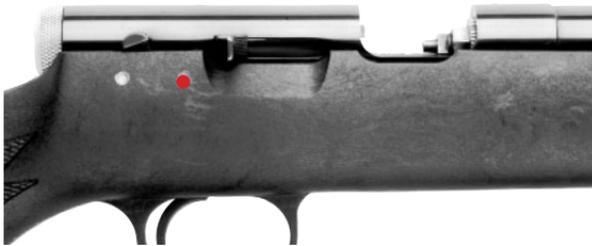
**Photo #2** Striker handle in the "Cocked" position with the thumb safety in the "Fire" position. The thumb safety will now be in line with the red dot in the stock. A pull on the trigger will now release the striker and cause it to strike the cap on the nipple.
