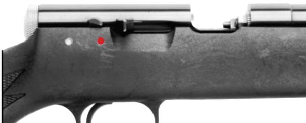
**Photo #3** The Striker handle in the "Fired" Position. The safety lever is fully forward and the Striker is also fully forward and in contact with the nipple.
