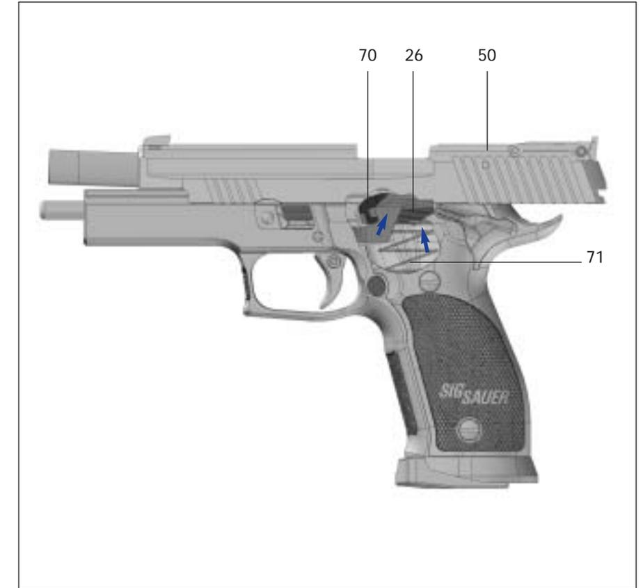
Fig. 21, slide is held open when magazine is empty
