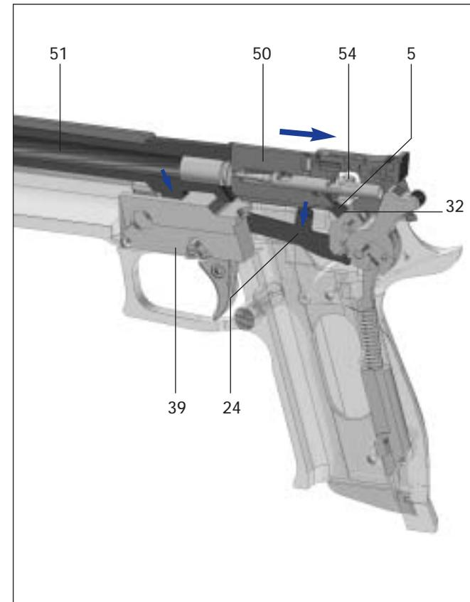
Fig. 19, barrel is tilted down and arrested
