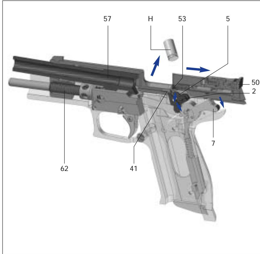
Fig. 20, case being ejected
