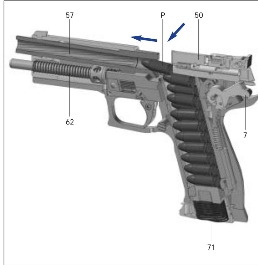
Fig. 15, round being chambered
