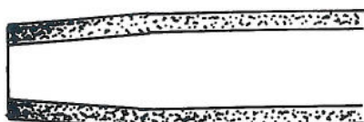
Swaged choke has been found on less expensive models. It is achieved by merely tapering muzzle of the gun.
