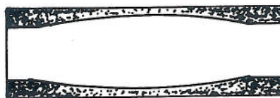
The so-called jug choke is made by hand with a rod, emery cloth. This is popular with Russian shooters.
