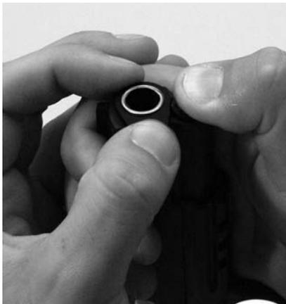
Figure 5: Rotating the barrel bushing
