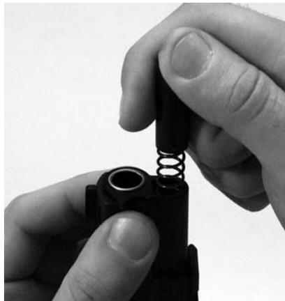
Figure 6: Releasing the recoil spring
