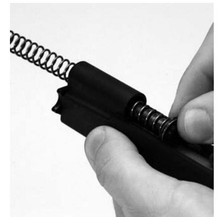
Figure 12: Insert recoil spring and guide into slide
