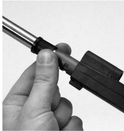
Figure 10: Removing barrel from slide
