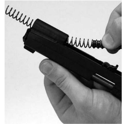
Figure 8: Removing recoil spring and guide
