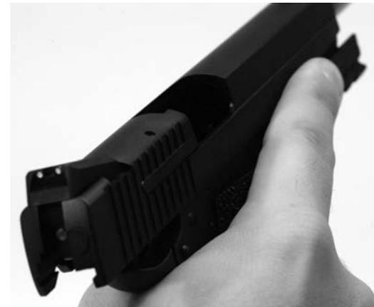
Figure 4: Visual check of the chamber
