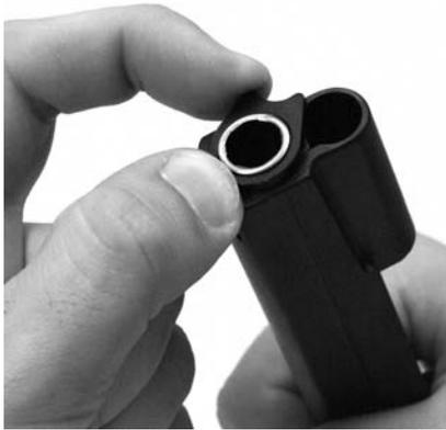
Figure 9: Removing bushing from slide
