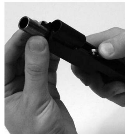
Figure 11: Insert barrel into slide
