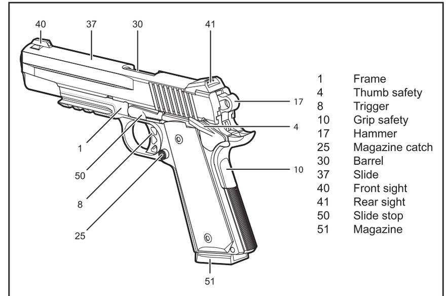
Figure 1: Pistol and magazine with major parts identified
