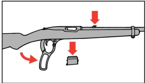
2. Loosen the barrel band screw (B-69) and remove the barrel band (L06801).
