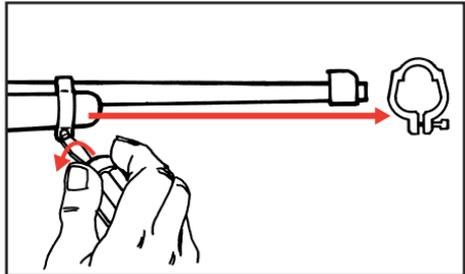
3. Loosen the take-down screw (L04701) completely, but note that it will not come out of the stock.
