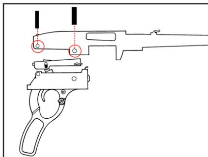
7. The bolt is separated from the lever by pushing out the bolt link pin (L04900).
