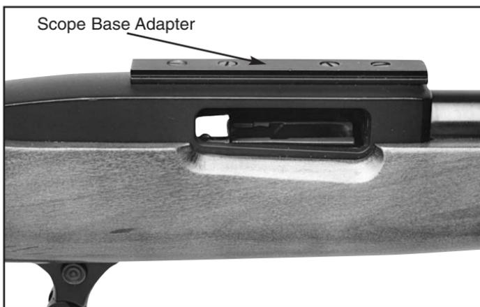
3. Position adapter on receiver and place a base-mounting screw in each hole of the adapter. Turn each screw until it just catches the threads in the receiver hole, but don't tighten the screws at this point.
