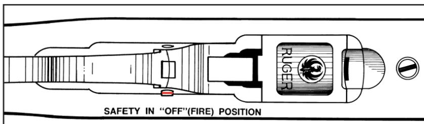
**Figure 2.** The underside of the trigger guard section of the rifle. In this illustration the safety is shown in the “off” (fire) position. The position of the safety and red band indicate the safety is “off.”
