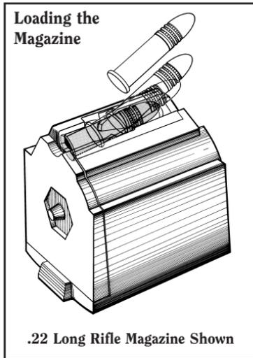
NOTE: The 9 shot Ruger .22 Magnum and .17 HMR magazines are **not** interchangeable with any other magazine. The .44 magnum magazines for the Ruger 96/44 lever action rifle and the Deerfield Carbine rifle will **not** fit into the Ruger 77/44 bolt action rifle due to dimensional differences. Do not attempt to use either of them in the Ruger 77/44.
