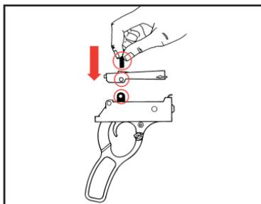
NOTE: Keep assembly level. Until the lever housing and receiver are reassembled, tipping the housing sideways may allow the bolt link pin to fall out of the bolt.
