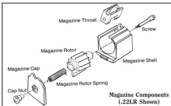
Exploded view of the magazine components. This illustration is included to show the relationship and names of the magazine components. As noted in the text above, the magazine should not be disassembled. The .22 Magnum, .17 HMR, and .44 magnum magazines are slightly different in dimension but are similar in concept and operation.
