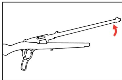
6. To remove the lever housing, again make sure the lever is fully open. Drift out the two larger diameter receiver pins with a small diameter screw driver or punch. Do not drive out any of the smaller pins. Do not disassemble the components of the lever housing assembly. The bolt is removed together with the lever housing.
