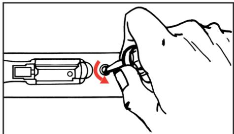
4. Position the safety so an equal amount of the button is exposed on each side. If the safety is not in the middle when the barrel-receiver assembly is lifted out of the stock, the stock will be damaged. Make sure the lever is open.
