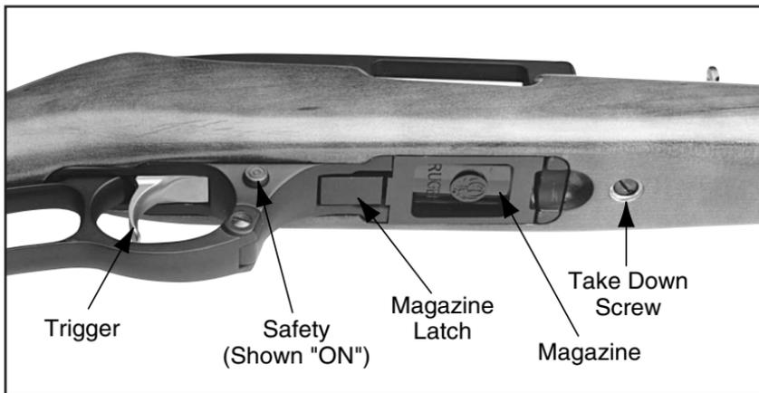
**Figure 1.** In these illustrations the frequently used operating components are identified. Note that the safety is protruding fully from the right side of the trigger guard and is therefore in its "on" (safe) position.
