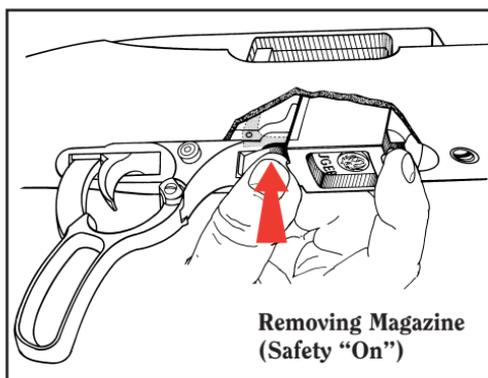
**Figure 3.** The lever should be open and the safety should be “on” when the magazine is being removed or inserted. When the forward section of the magazine latch is pushed in (pivoted upward), the magazine is released. Depress the latch with the thumb and at the same time grasp the magazine between the thumb and forefinger and draw it out of the rifle.
