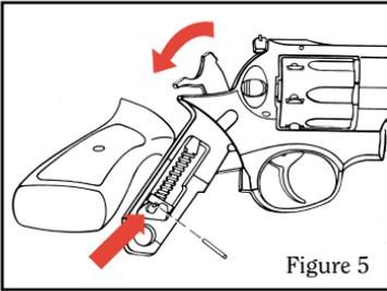
2. Using a properly fitting screwdriver, remove grip screw. Remove pistol grip inserts from grips. Grip panel locator may then be removed. Pull grip downward off frame. Take care not to lose the disassembly pin, which may fall free when the grip is removed.
