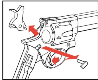
5. Pull trigger and remove hammer pivot while holding trigger in a rearward position. Lift hammer out of the top of the frame while trigger is held in a rearward position (See Figure 6).
