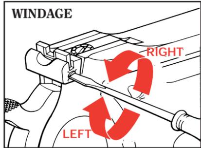
To move the point of impact to the right: turn screw counterclockwise.
