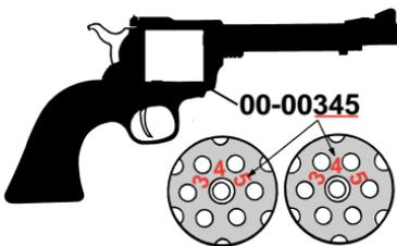
Do not accept delivery of a New Model Blackhawk Convertible (a model with two cylinders) unless the numbers on the front face of both cylinders match the last three digits of the serial number on the frame. Use of the wrong cylinder can cause improper alignment or timing and may result in personal injury.
