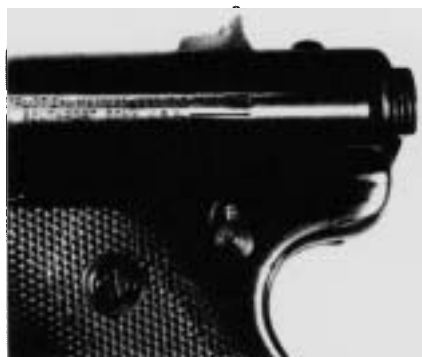
Figure 5. Safety shown in "fire" (F) position. Safety is all the way down .
