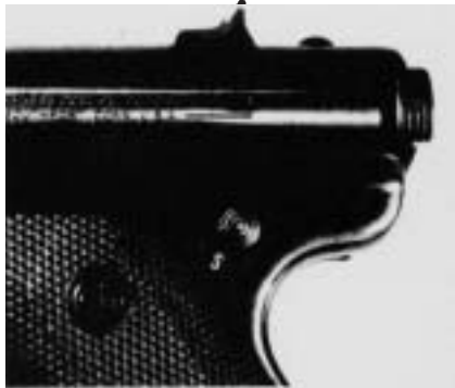
Figure 6. Safety shown in "safe" (S) position. Safety is all the way up .
