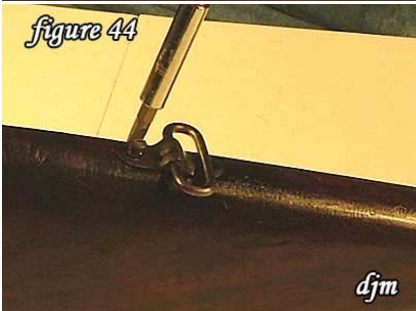
44) Unscrew the rear rear swivel screw.
