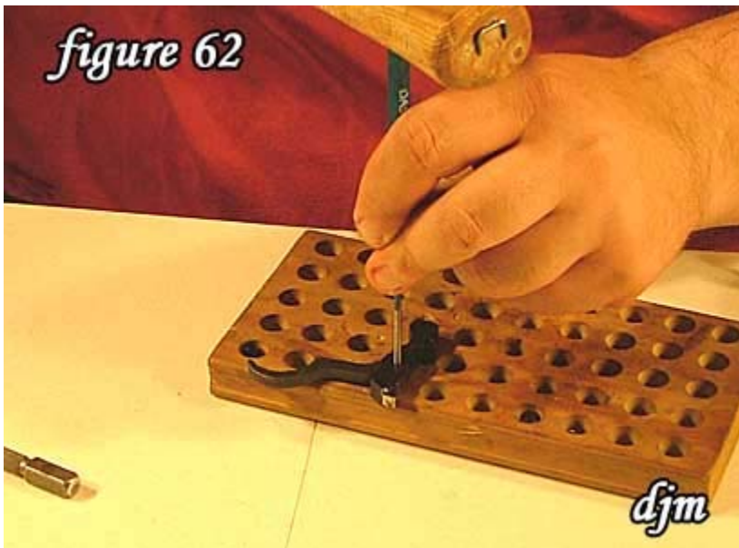
62) Tap trigger pin into place.
