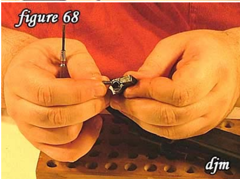
68) Insert plunger spring into cut-off.
