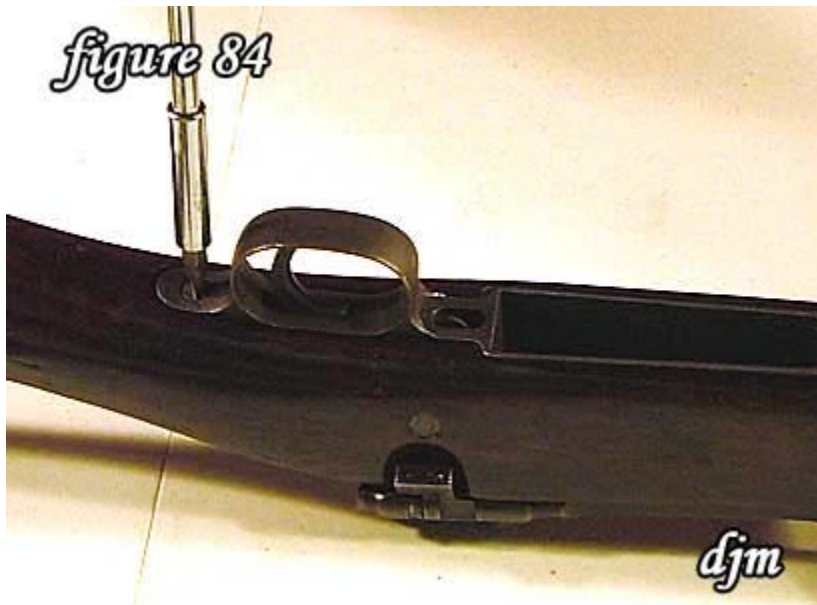
84) Fully tighten the rear guards screw.
