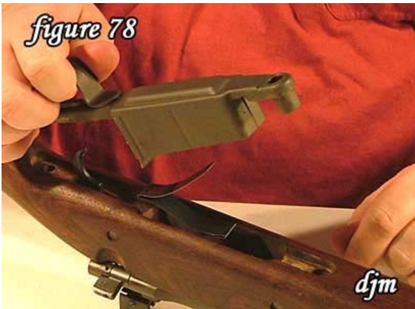
78) Figure 78 shows the 03A3 and 03A4 stamped metal trigger guard (with non-removable floor plate) being installed into the rifle.
