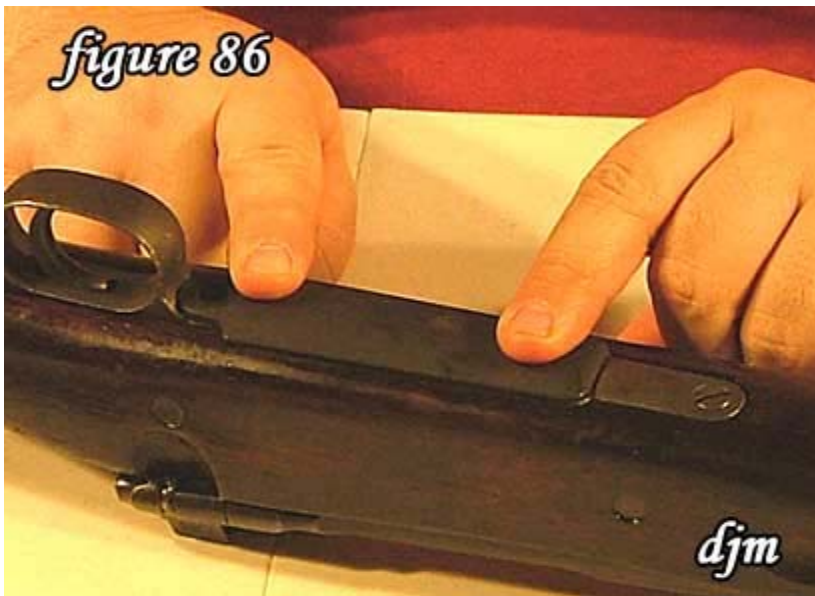
86) (1903 and 1903A1) Snap floor plate in place.
