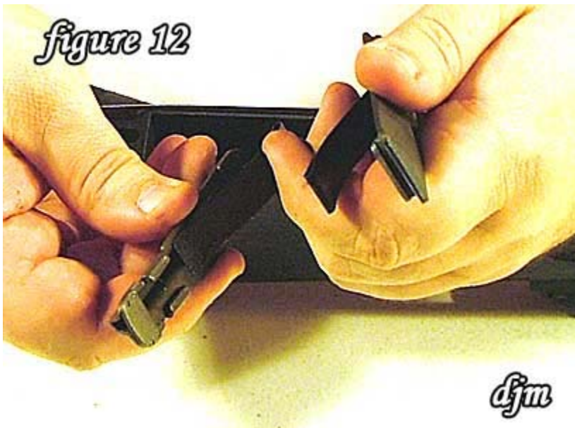
12) Separate follower from magazine spring.
