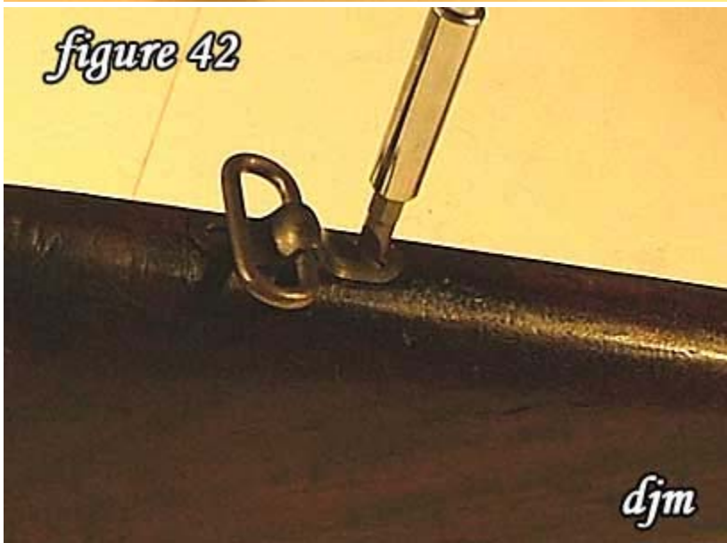
42) Unscrew the front rear swivel screw.
