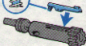
2 Insert extractor and spring
