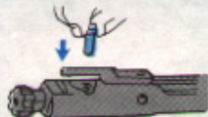
5 Replace bolt cam pin
