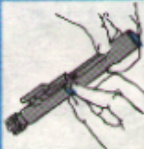
8 Replace retaining pin
