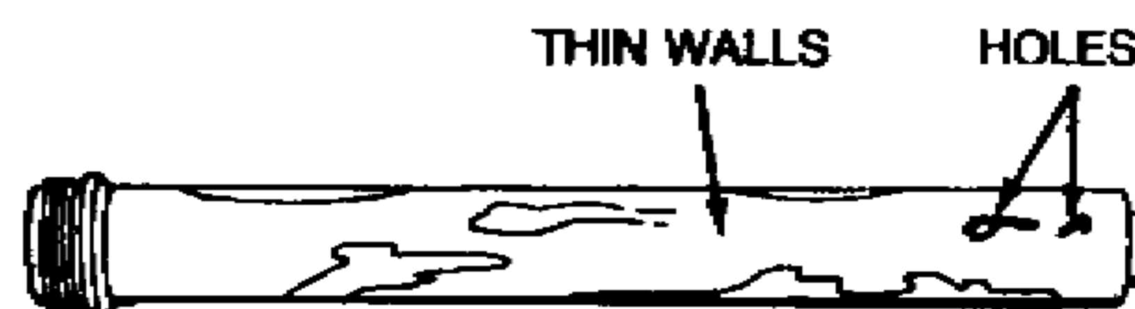
HOLES AND THIN WALLS
