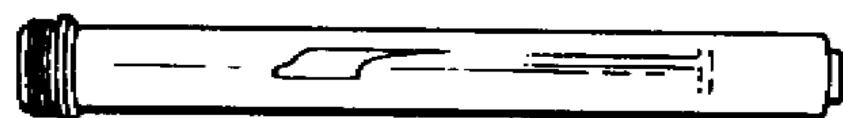
SHINY SURFACES (REPARABLE)
