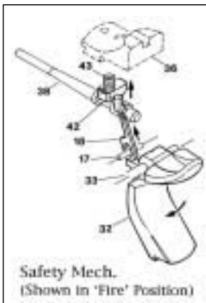
If your Kimber is a Series II firearm, then it is supplied with an integral firing pin block. This feature does not allow the firing pin to be active until the Grip Safety is depressed. **THIS ADDED SAFETY DOES NOT ELIMINATE THE NEED FOR SAFE AND PROPER GUN HANDLING. READ THIS OWNERS MANUAL THOROUGHLY.**
