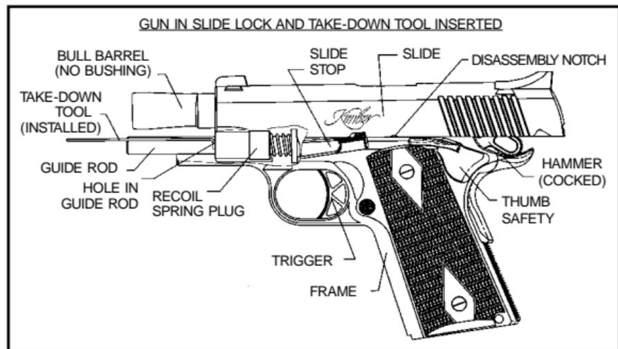
2. With hammer still cocked, push the slide forward until the semi-circular tab on the back of the slide stop aligns with the semi-circular disassembly notch in the bottom of the slide.
