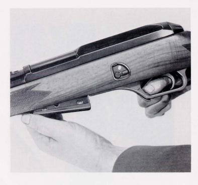
Remove the magazine by pressing the magazine catch. Retract cocking lever quickly, tilting the rifle somewhat to the side to permit a round that might be left in the chamber to slide out of the ejection port into your hand. Close the rifle and pull the trigger. The rifle is now unloaded and uncocked.
