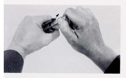
Rotate the bolt head clockwise one quarter turn, and then remove it from the locking piece. Finally, remove locking piece, firing pin and firing pin spring from the bolt head carrier by rotating the locking piece further.
