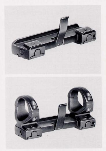
Our HK 05 clamp mount readily accepts all standard telescopic sights. Should you wish to use an aluminium rail-type telescopic sight, loosen the two hexagon socket screws on the bottom of the 05 clamp mount, slide on the telescopic sight and tighten the two hexagon socket screws firmly at the rails. If you are using a steel telescopic sight, please also use the retaining rings.
