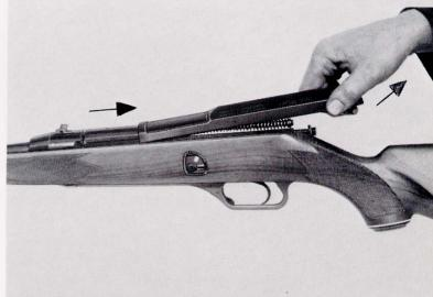
You can now remove the bolt assembly by passing a screwdriver through the hole for the screw and forcing the firing pin forward. It is not necessary to further strip the rifle for cleaning (except for the bolt assembly).
