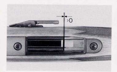
the bolt head carrier. You can determine this, if you can put a sheet of paper between bolt and bolt head (see fig., gap >0). If this gap has disappeared, please have the weapon checked by your local gun dealer as this technical condition would cause excessive strong recoil forces and thus damage the bolt system.
