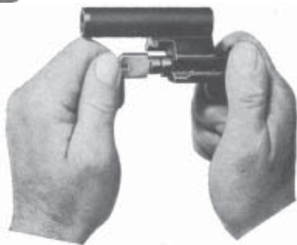
Fig. 38 Stripping the bolt assembly
