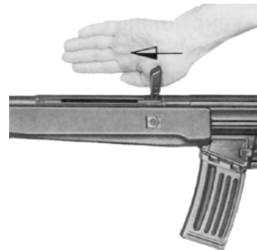
Fig. 33 Releasing the cocking lever
