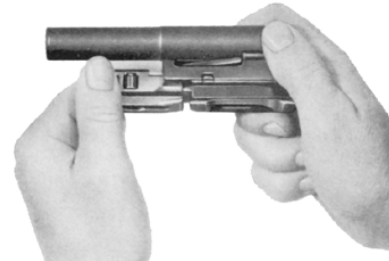
Fig. 38 Stripping the bolt assembly
