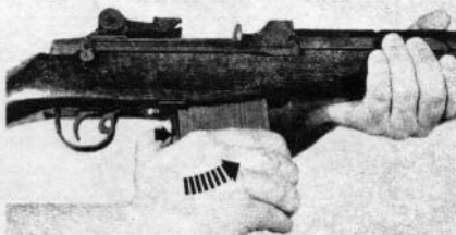
Figure 4. Removing the magazine.
