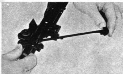
Figure 17. Replacing the connector assembly.
