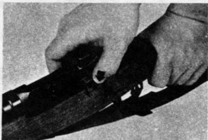
Figure 5. Locking the bolt to the rear.
