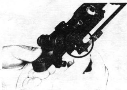
Figure 13. Removing operating rod.
