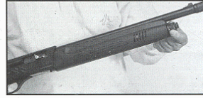
Fig 5: Slide the forend over the magazine tube (do not force). Make sure that the forend is completely seated around the magazine tube, barrel, and the receiver (note the forend has two plastic notches that interlock into the receiver).
