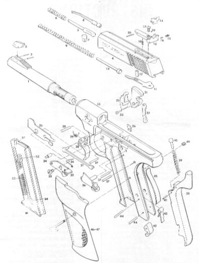
Main spring housing will snap out at the bottom and can be removed along with the sear spring. Remove slide and magazine. The pistol is now ready for cleaning.
