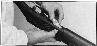
Fig. 7: Turn the shotgun upside down so that the barrel is pointing toward the ground and you are looking at the carrier latch. Now depress the carrier latch
