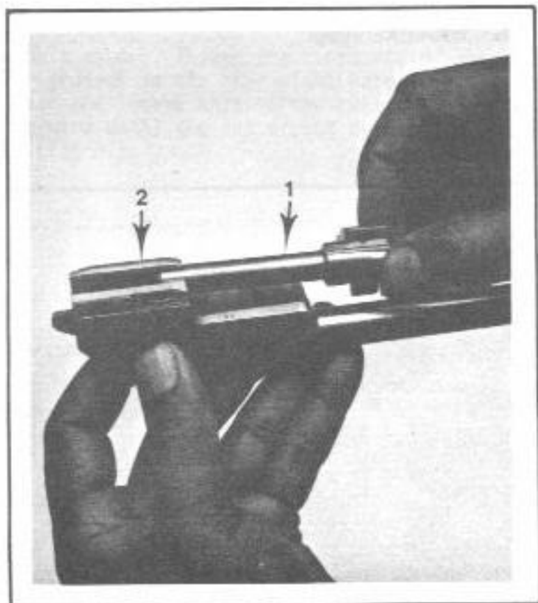
FIGURE 38. REPLACING THE BOLT
