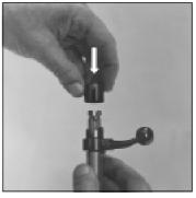
Replace the sleeve and make sure that the slot in the sleeve lines up with the firing pin lug.
