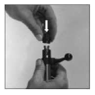
Replace the safety with the signal pin and spring and make sure that the safety wing lines up with the firing pin lug and that the signal pin is properly seated.
