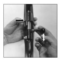
Depress bolt stop on left side of receiver and pull bolt out to the rear. This removes the bolt from the receiver.
