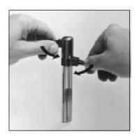
Hold the bolt as shown and turn the bolt handle clockwise and the wing safety counter-clockwise as far as they will go.
