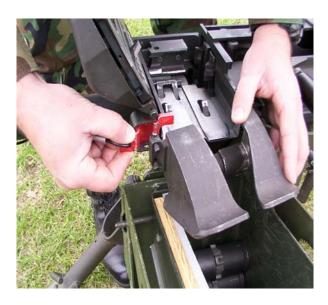
D. Unscrew the AR-22 barrel insert from the yoke.
