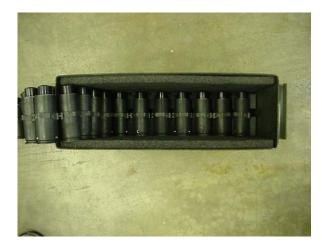
(Note: One end of the foam tray at the bottom of the ammunition can is higher than the other end. The high end must be placed to the *right*. The male end of the belt rests next to this high end. The large panels of foam must be at the sides of the ammunition can.)
