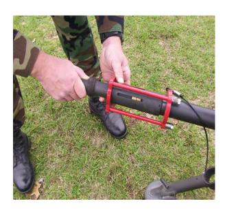
F. In cool weather, water from propellant gasses may condense on the insert or Mk19 barrel. Wipe them clean and dry, then oil them to prevent damage to either.
