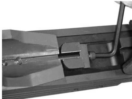
Figure 15 Loosening the Bedding Wedge
