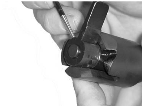
Figure 14 Disassembling the Bolt Sleeve and Striker Group
