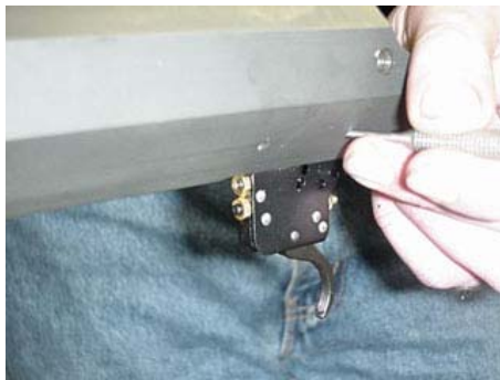
Figure 19 & 20 Removing the Trigger Group
