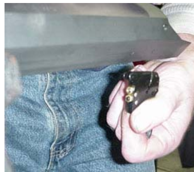
Figure 19 & 20 Removing the Trigger Group
