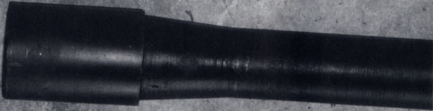
Breech end of barrel with locking lug section in place.
