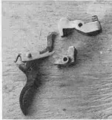
Component parts of trigger assembly.
