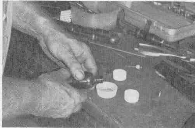
Acid is poured into small plastic cups. Only a small amount is required.
